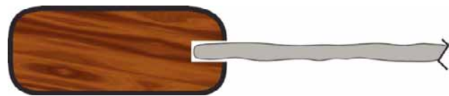
Specialized mouldings for stained glass have a dado rather than a rabbet. Their appearance is the same on both sides, important if it is to hang in a prominent window where the outer side is easily seen.
