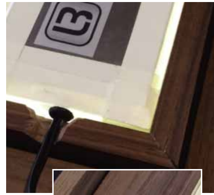
The only modification needed for the LED panel was a small notch cut into the frame for the power cord, and this was accomplished in less than a minute with a Dremel rotary tool.
