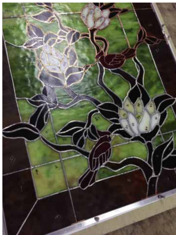
Stained glass worked in the Tiffany method midway through the soldering process. Once the soldering is complete, a small metal frame is applied, the solder has a patina applied, and the entire piece is cleaned and polished.
