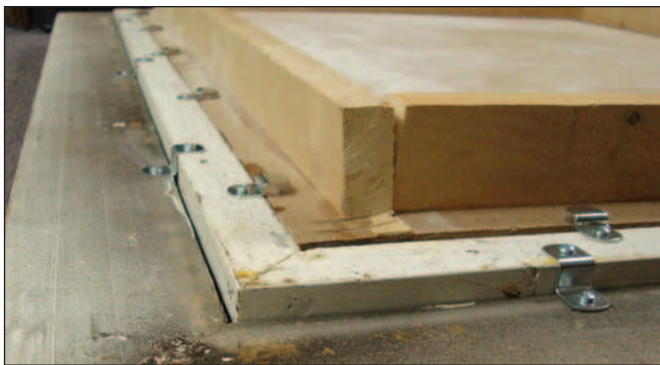
The lifter is spread at the corners due to warping of the panel.
