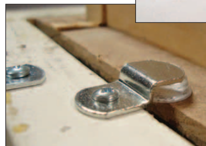
In this example, the top end is screwed to the frame while the bottom end is pressing the backed canvas to hold it.
