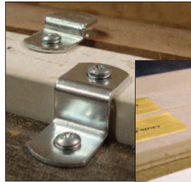
In this example, the top end is screwed to the frame while the bottom end is pressing the backed canvas to hold it.
