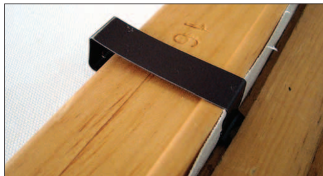
These commercial canvas clips are mounted in shallow wood rabbet.
