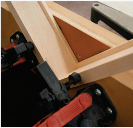
● The frame must begin with an accurate miter so there are no gaps in the joint.
