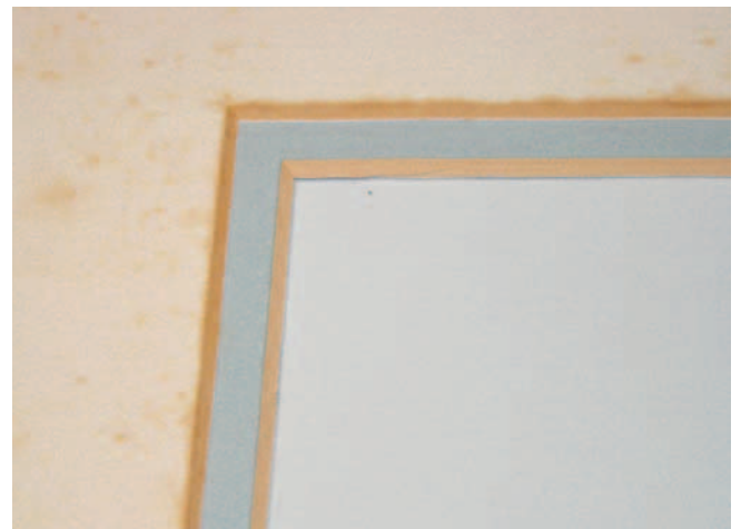
A decorator-grade matboard that was originally marketed as “acid-free,” revealing the long-term results of buffering saturation and subsequent acid burn.
