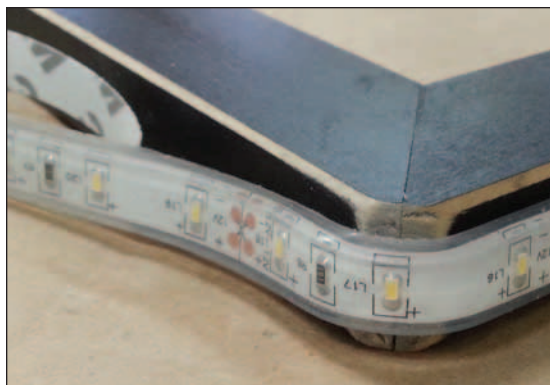
(Above) A strip of LED lights was wrapped around the original black frame, now with rounded corners. (Below) The back of the finished frame shows the hanging hardware, spring clips holding on the backing board, and the wiring going to the LED lights.
